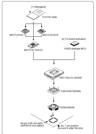
Figure 2 Usage of the M3T-100LCC-80QSB
